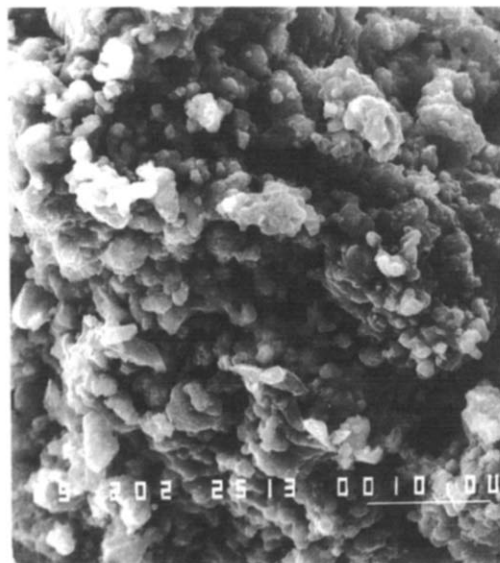
Fig. 4. Mechanochemically synthesized TiB 2 particles ( \times 2000 ).
